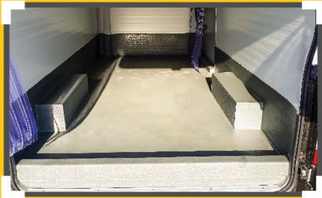
1 Ton Pick-up/Van PU Coating. The floors use polyurethane coating, which is antifungal, and ensures no water leakage; such floors are easy for cleaning too, and are needed for products as specified by the Food Control Division of the Municipality.
